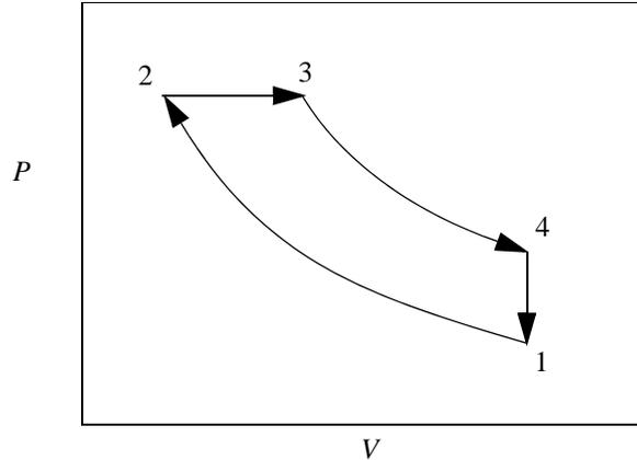
Figure S-5.4 Schematic of air-standard Diesel cycle.
