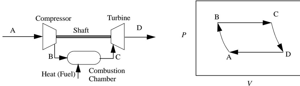
Figure S-5.1 Gas turbine, and schematic of air-standard Brayton cycle.
