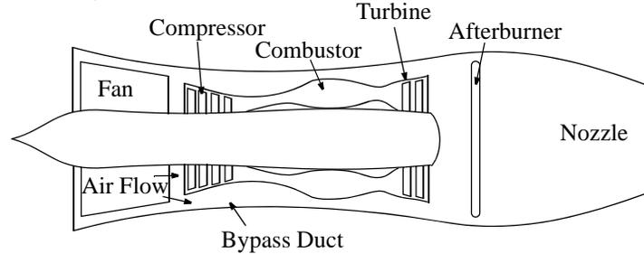
Figure S-5.2 Schematic of a typical turbofan jet engine.
