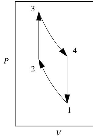
**Figure S-5.3** Schematic of the air-standard Otto cycle.
