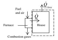
$$\frac{d}{dt}(mU) = \underline{Q}_{gain} + \underline{Q}_{loss}$$
