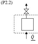
Before the valve is stuck,  $\Rightarrow$  there is steam escaping and therefore, there is an enthalpy for the vapor leaving, no expansion / contraction work, no shaft work, no kinetic or potential energy occurred.
